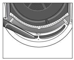
Use a vacuum cleaner with a long crevice nozzle attached to remove any visible fluff from the upper air flow openings.
